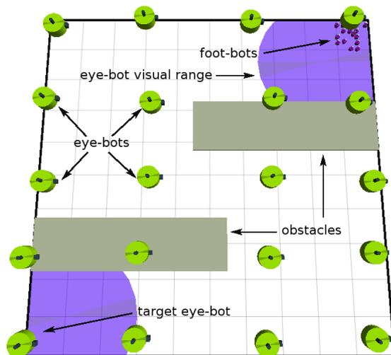
**Fig. 2** Example problem scenario. The foot-bots are deployed in the start location at the top right of the arena. The target location is at the bottom left. The eye-bots take positions against the ceiling in the area between source and target.
