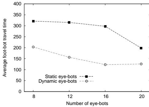
**Fig. 13** Results of experiments with randomly placed eye-bots in the scenario of Figure 2: average foot-bot travel time ( $t_a$ ) vs. number of eye-bots.
