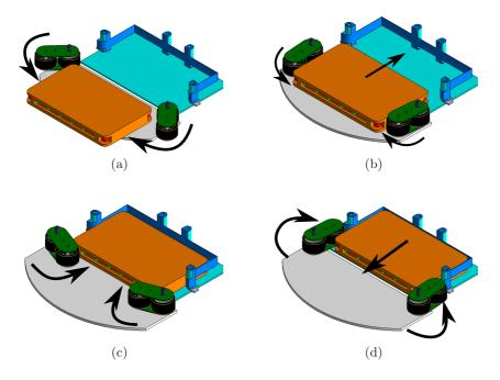
**Fig. 2.** (a) The arms rotating towards a *book-bot* on the loading bay. (b) The wheels pushing the *book-bot* inside a slot. (c) The arms finishing to push the *book-bot* in the slot. (d) The arms reversed to get a *book-bot* from a slot.
