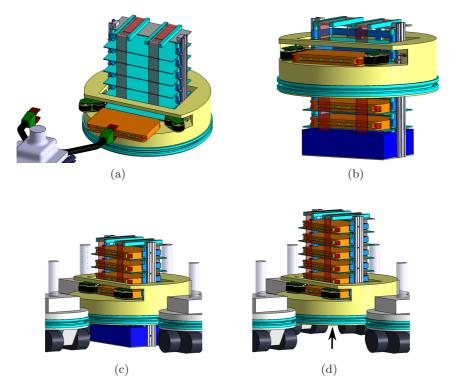
**Fig. 1.** (a) *Book-bot* put on the loading bay by a *hand-bot*. (b) Base elevation on the rack to reach a high slot. (c) *Foot-bots* docked to the *cart-bot*. (d) Rack elevated to remove friction with the ground.
