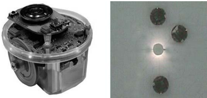
Fig. 1 Left : The e-puck robot developed at the Swiss Federal Institute of Technology in Lausanne (EPFL) (Mondada and Bonani 2007). Right : A close up view of the environment with the light bulb in the centre and three robots
