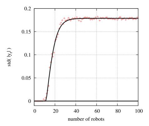
Figure 14: Average standard deviation of the absolute value of the  $y_r$  position for each s-bot r, plotted varying the group size R from 1 to 100. The black line represents a curve that fits the experimental data.
