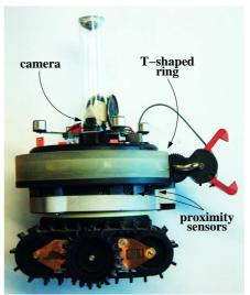
Figure 3: View of the s-bot from different sides. The main components are indicated (see text for more detail).
