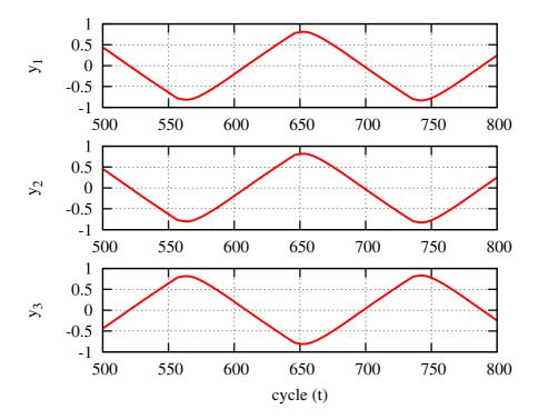
Figure 2: An example of synchronised motion of three robots. The y position of the robots is plotted against time.
