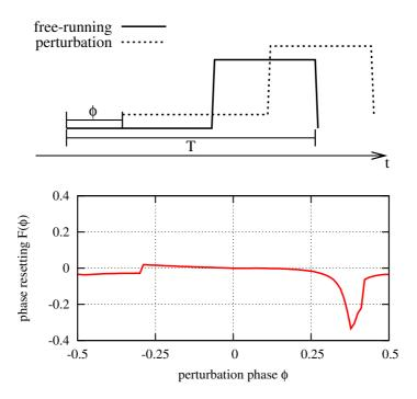
Figure 8: Top: Definition of the perturbation phase  $\phi$  from the time delay between the signal of the free-running oscillator and the perturbation signal. Positive values correspond to a delayed signal, while negative values correspond to an anticipated signal. Bottom: Normalised phase response curve (PRC) for controller  $c_8$ .
