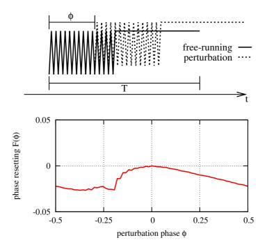
Figure 10: Top: Definition of the perturbation phase  $\phi$  from the time delay between the signal of the free-running oscillator and the perturbation signal. Bottom: Phase response curve for the controller  $c_{10}$ .
