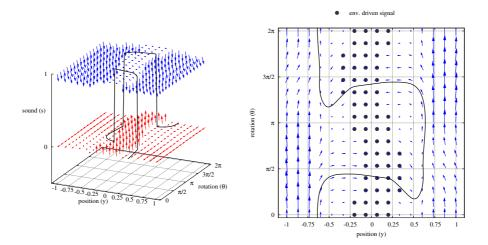
Figure 13: Individual behaviour of controller  $c_{13}$ . Left: the 3D vector field shows for each point in the phase space the direction of variation and its magnitude. Right: projection on the  $y\,\theta$  plane of the vector field for a constant perceived signal s=1. The black line represent the limit cycle for this condition. The black dots represent the non-interaction area.
