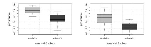
Figure 15: Comparison between the performance obtained in simulation and with physical robots.
