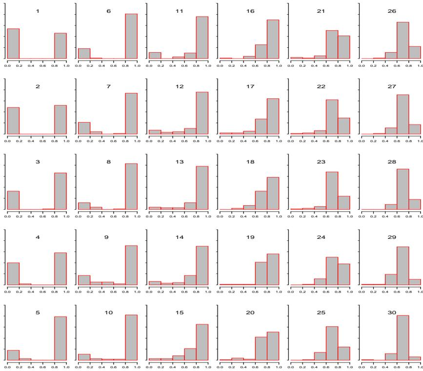
**Fig. 10** Frequency histogram (over 100 test runs) of the path selection ratio  $\rho$  in the scenario of Figure 9 for the number of foot-bots ranging from 1 to 30. The y-axis scale of all plots ranges from 0 to 1.
