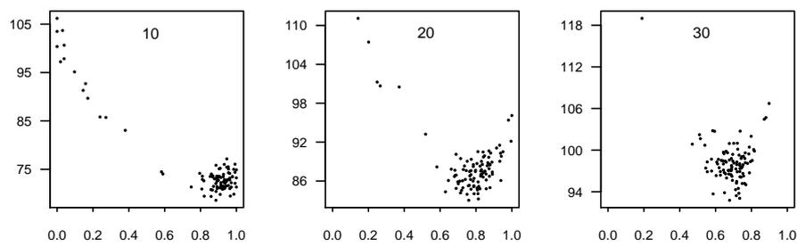
**Fig. 11** Scatter plot of the path selection ratio  $\rho$  versus the average time needed by foot-bots to travel between source and target,  $t_a$ , for the tests with 10, 20 and 30 foot-bots.
