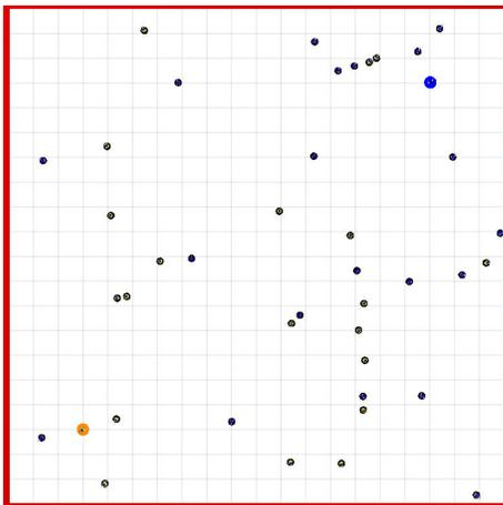
Fig. 4. Setup for swarm navigation experiments. The area is 20x20 m<sup>2</sup>. The target robots are located in the top-right and bottom-left corner (indicated with large orange and blue disks).
