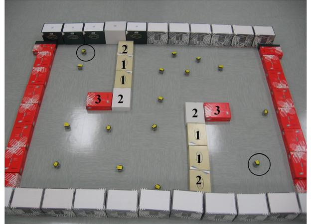
Fig. 6. Scenarios of increasing difficulty for the real robots: scenario 3 includes all boxes labeled 1 up to 3, scenario 2 includes the boxes labeled 1 and 2, and so on. The robot indicated with a circle in the bottom right is the searcher, and the one in the top left is the target.
