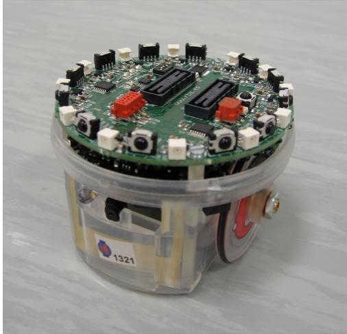
Fig. 5. An e-puck robot with IrRB module.
